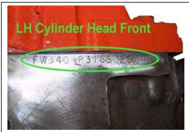
Engine: Build location, CID, build date and total engine built that day
