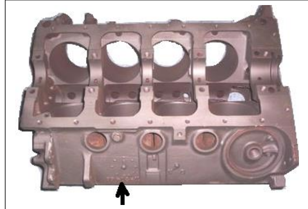
Reference 1970 340 engine casting date and manufacturing date wheel location on the RH side of the block
